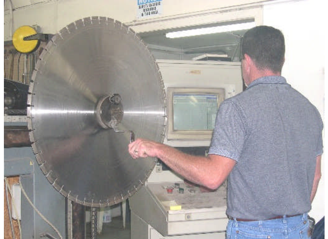
BLADES ARE TENSIONED
